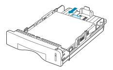
3 Pinching the paper width guide as shown, move it toward the stack of paper until it lightly touches the side of the stack.
